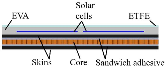
Figure 1: Sketch of lightweight PV module design for BIPV applications.
